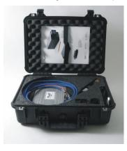
The miniLDV system includes a miniLDV probe, driver electronics, band-pass filter, and BP-miniLDV acquisition hardware and processing software (computer and traverses are optional).
