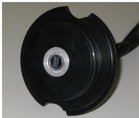
The microV probe is easy to incorporate into flow models with its small size, simple geometry, and rugged construction.
