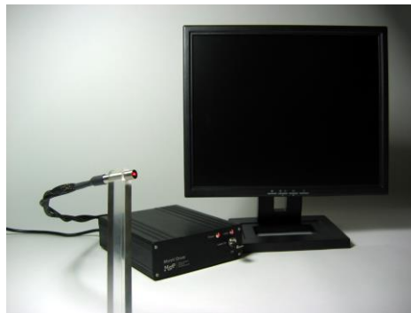
The microV System consists of a microV probe, driver electronics, and BP-microV acquisition hardware and processing software (computer and traverses are optional).
