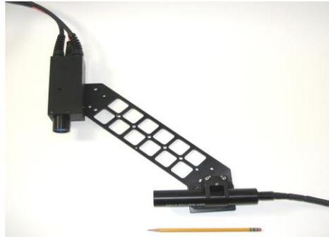
*The 3D miniLDV probe is extremely compact, self contained, and permanently attached to a structure; no calibration or alignment by the user is required. The probe contains three high power lasers, miniature beam shaping optics, and detection optics.*
