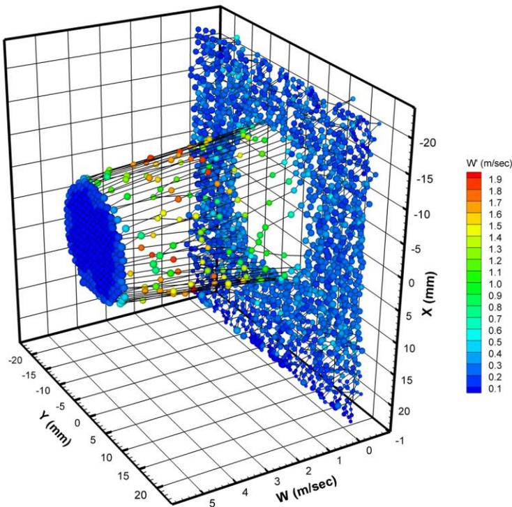
Above: the out-of-plane component of velocity in the cross section of a turbulent jet near the nozzle exit, automatically collected in less than 2 hours by *BP-miniLDV* software. The measurement was collected in the 2-by-2-inch test section of the flowLab facility – the measurement would have been difficult with a Stereo PIV system. (Color corresponds to the RMS value of the out-of-plane velocity.)
