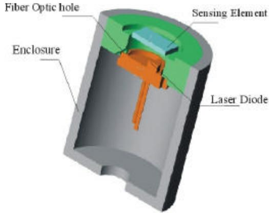
**Figure 10. Shear stress sensor assembly.**
