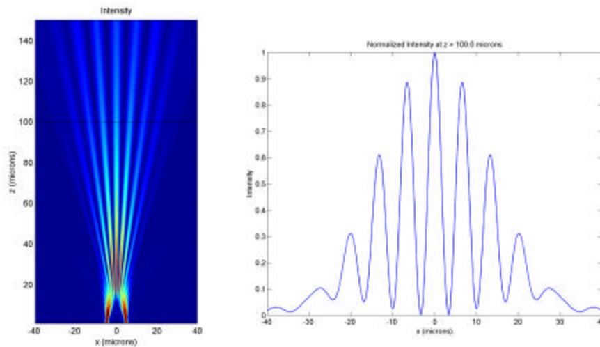
**Figure 8. Fringe pattern resulting from 2 μm slits separated by 10 μm (propagation of a finite-difference solution of slit diffraction when illuminated by the dual-line-focus laser lens).**
