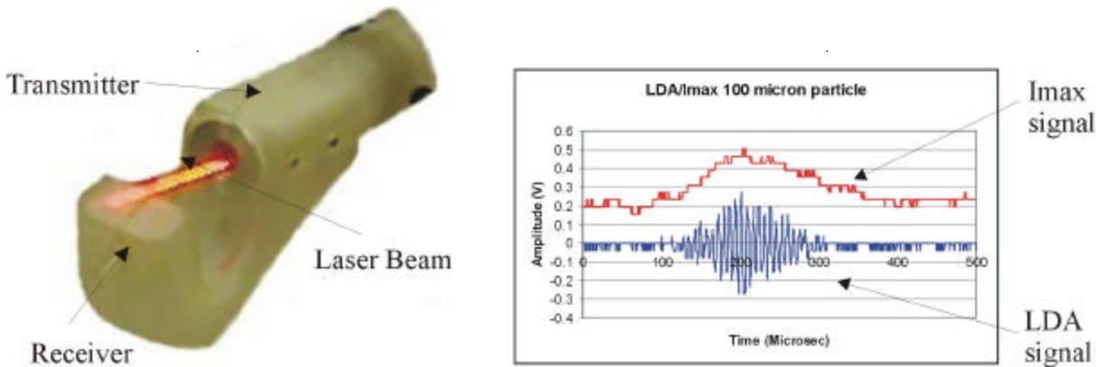
Figure 12. Particle sizing device and sample signal trace.
