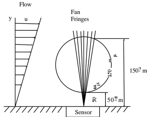
Figure 6. Schematic of the shear stress sensor principle.
