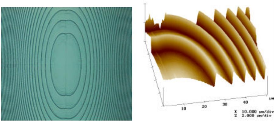
**Figure 9. Photograph (left) and AFM scan (right) of the center of the dual-line-focus laser lens**
