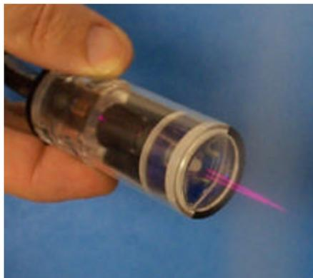
**Figure 1. Photograph of a miniature laser Doppler anemometer.**
