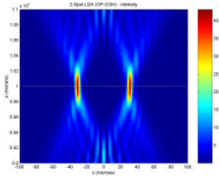
**Figure 5. Modeling results of the fringe pattern generated by computer-generated-hologram grating coupler.**
