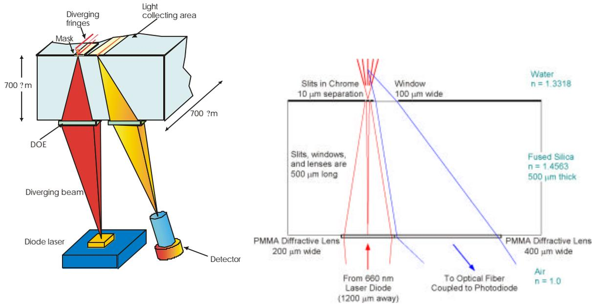
**Figure 7. Schematic of the shear stress sensor assembly.**
