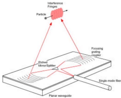
**Figure 3. Conceptual design of the integrated optics micro-LDA.**
