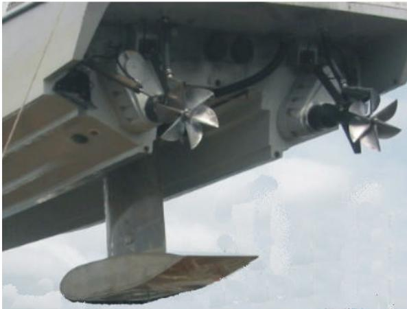
**Figure 10 - SDV 45 ft boat with the attached hydrofoil**
