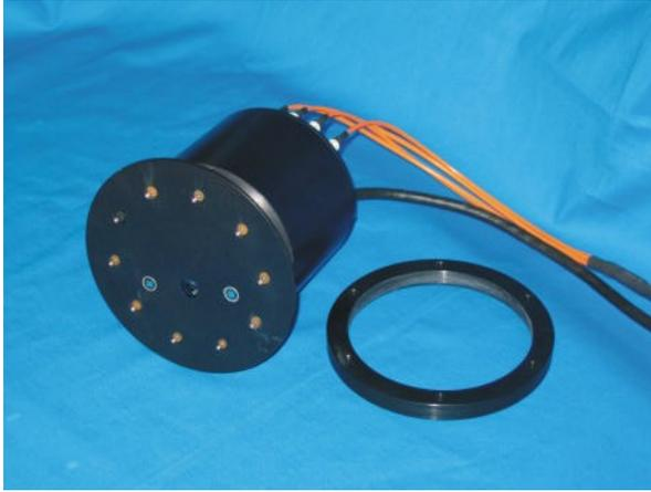
**Figure 9 - Multi-location Velocimeter Package used at SDV45**
