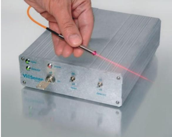
**Figure 6 - Cross-Correlation Velocimeter Probe and Power Supply**
