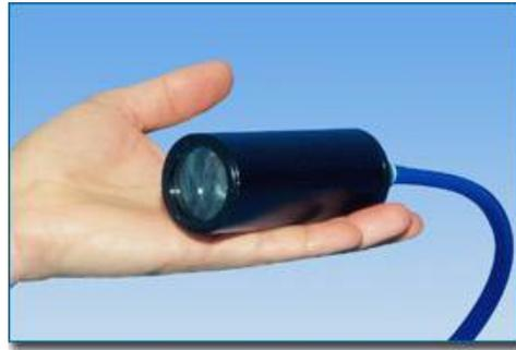
Figure 2: Photograph of the MiniLDV probe (Measurement Science, CA)
