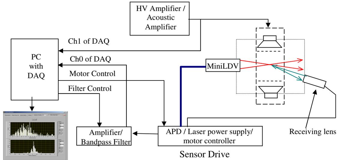
Figure 4: Schematic showing the basic setup of the Dust Particle Analyzer (DPA)
