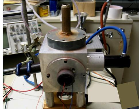
Figure 3: DPA relaxation chamber for Mars simulant dust sampling.
