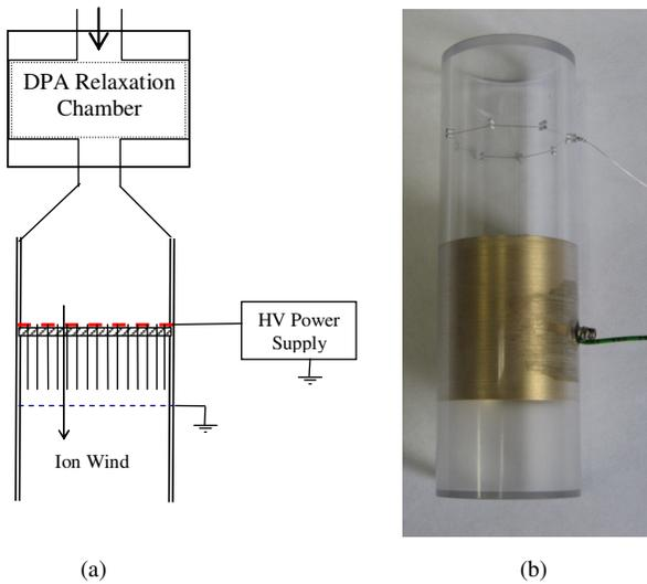
Figure 5: Schematics of the two types of EHD pump for sampling Mars atmospheric dust particles through the DPA relaxation chamber.
