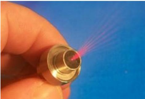
Figure1 : Image of the MicroS3 shear-stress sensor.
