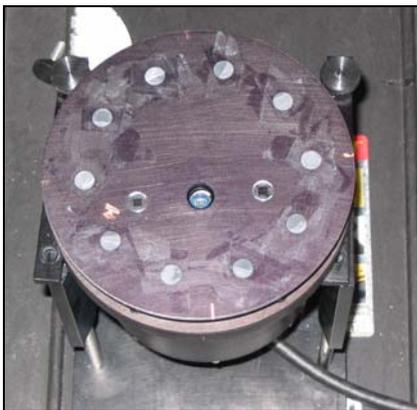
**Figure 18- Integration of two MicroS shear stress sensors with a traversing microV for boundary profilometry within 2mm from the surface**
