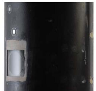
*A custom cylindrical enclosure containing a traversing miniLDV and two microS for flow separation studies.*
