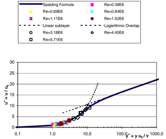
**Figure 11 Spalding fit to dual velocity measurements using the Dual Velocity sensor**
